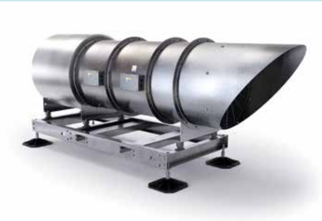
AXTÂN ASSEMBLY WITH INLET SILENCER Horizontal Skid Assembly Certified to EN12101-3. 800mm dia. Smoke Run & Standby axial with exhaust cowl, backdraft damper, room side silencers, matching flange, and flexible connector. Code: AXH80DG-4LR
