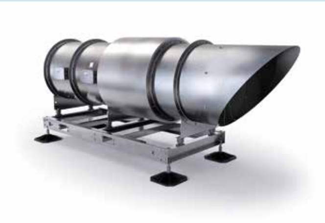
AXTÂN ASSEMBLY WITH OUTLET SILENCER Horizontal Skid Assembly Certified to EN12101-3. 800mm dia. Smoke Run & Standby axial with exhaust cowl, backdraft damper, atmosphere silencer, matching flange, and flexible connector. Code: AXH80DG-4LA
