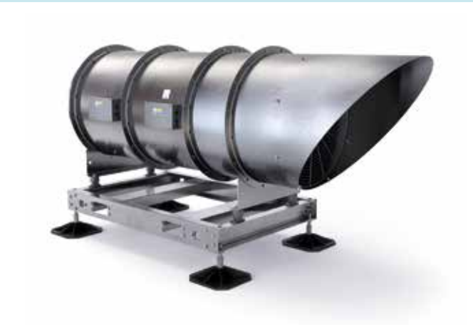
AXTÂN ASSEMBLY WITHOUT SILENCERS Horizontal Skid Assembly Certified to EN12101-3. 800mm dia. Smoke Run & Standby axial with exhaust cowl, backdraft damper, matching flange, and flexible connector. Code: AXH80DG-4LN
