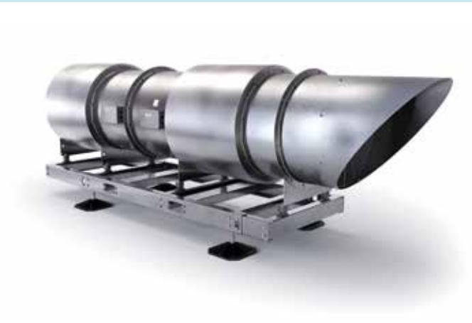
AXTÂN ASSEMBLY WITH INLET & OUTLET SILENCERS Horizontal Skid Assembly Certified to EN12101-3. 800mm dia. Smoke Run & Standby axial with exhaust cowl, backdraft damper, room side and atmosphere silencer matching flanges and flexible connector. Code: AXH80DG-4LB
